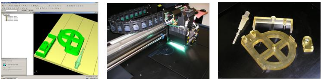
Figure 2. Three stages of additive manufacturing by Objet Eden 350V machine: preparing geometry in electronic format (STL) and importing it into the slicing software, manufacturing, models printed after cleaning
