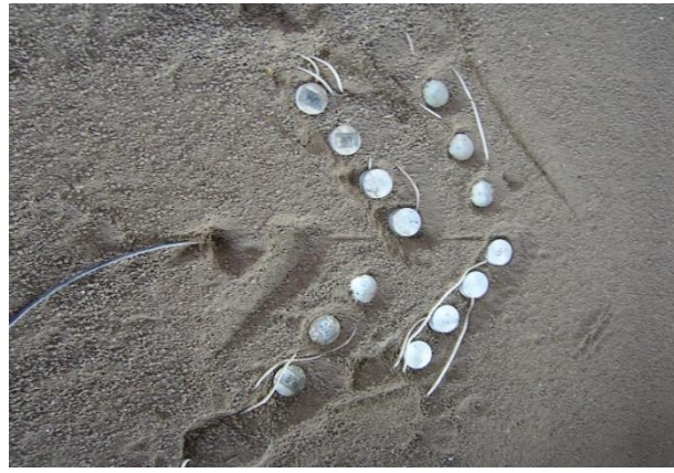
Figure 7. Placement of sensors under the tyre
