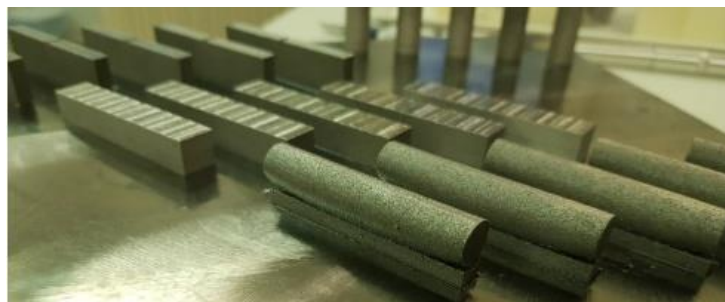
Figure 6. Cuboid and cylindrical test specimens produced by the SLM machine in horizontal and vertical orientation
